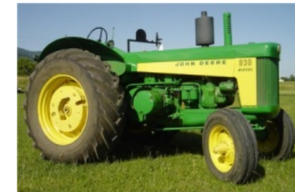
1958 - John Deere 830 7.5-18 / 18.4-34 250/80 kPa 56 kW
