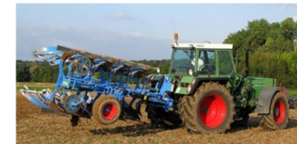
1976 - Fendt 614 SL 16.9R26 / 20.8R38 130/100 kPa 100 kW
